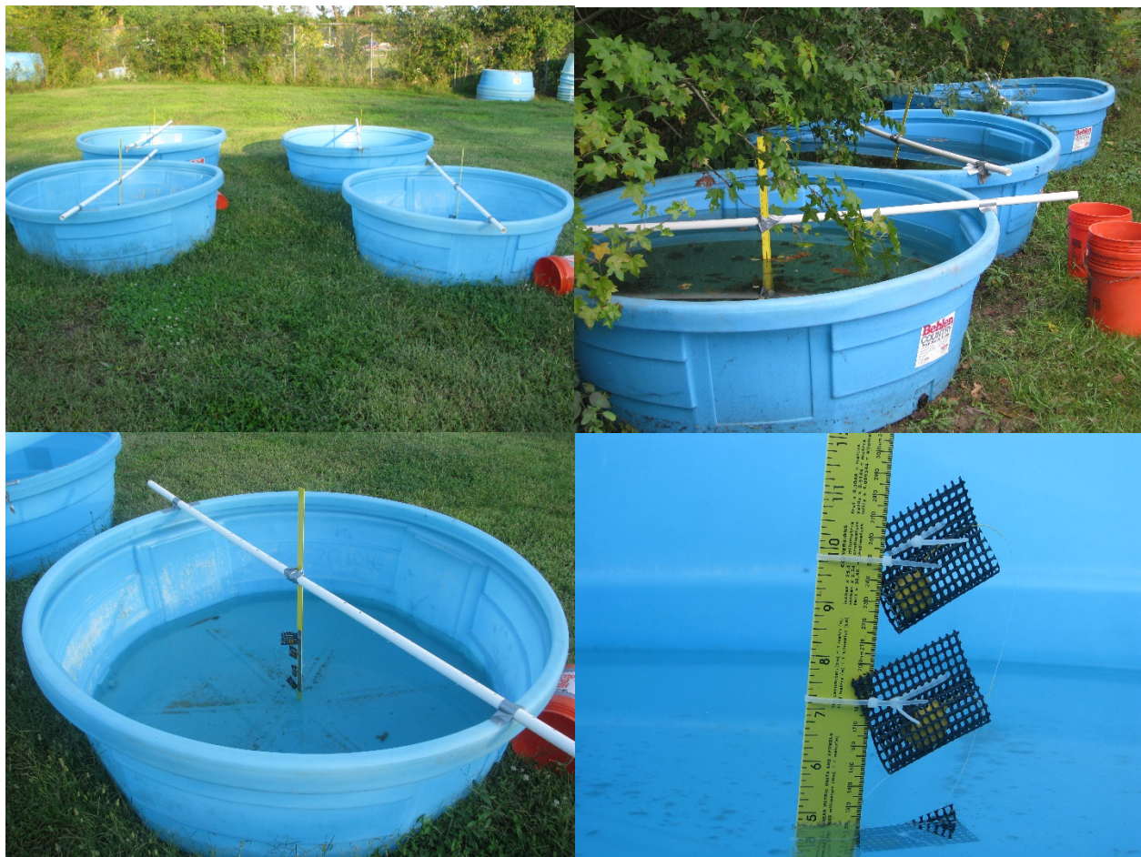
Figure B1: Experiment 2 set up and design. The top two panels are the open (top left) and shaded (top right) treatments, and the bottom two panels show iButton attached and set up.
